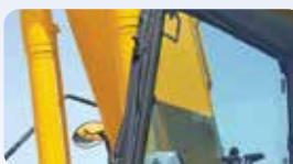
Remote intermittent wiper with windshield washer
