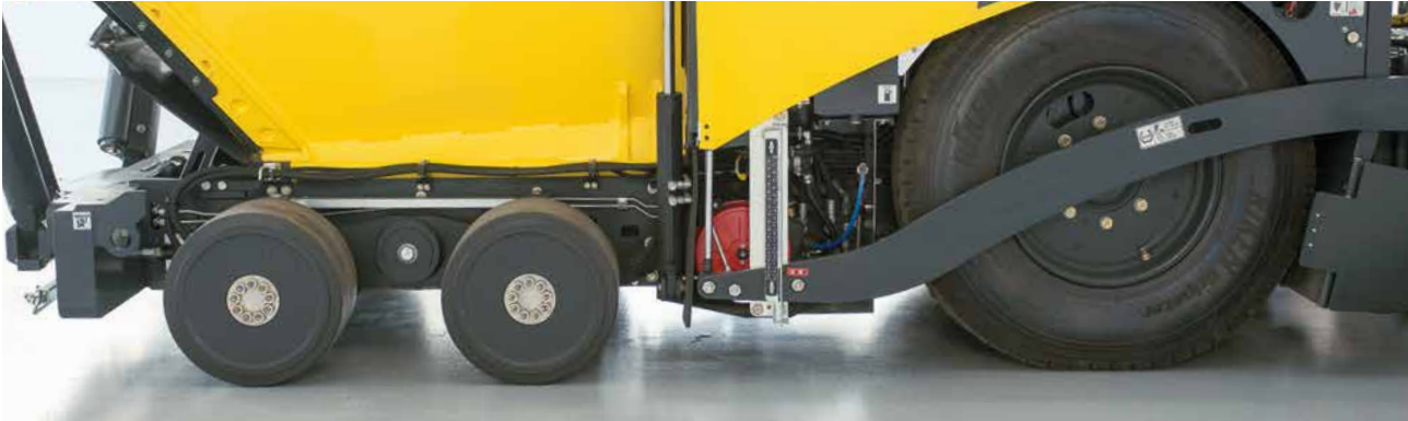
Optional 6 x 6 wheel drive for maximum tractive force.
