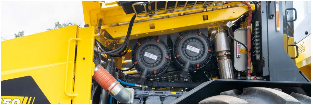
TIER 4 final / Stage 5 with double SCR system.
