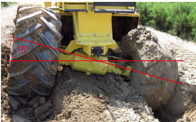
Non-spin oscillating axle +/- 15°.
