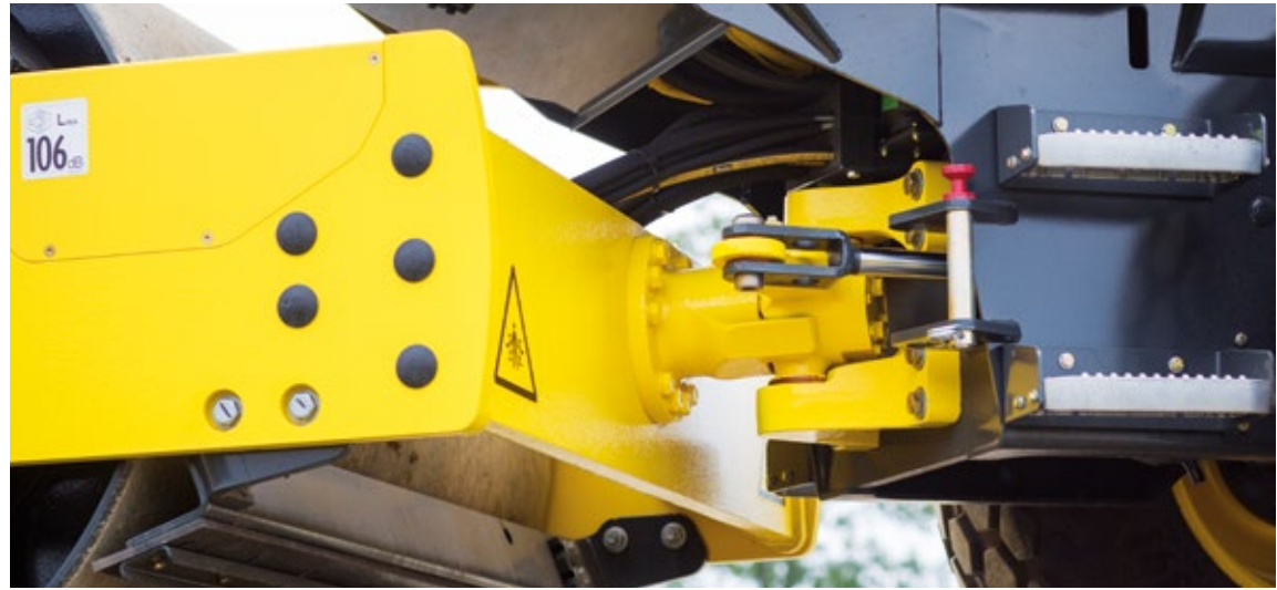
Cleanly executed: The articulated joint is maintenance-free; the machine needs no lubrication whatsoever.
