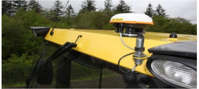
Increasing precision: the BOMAP GPS antenna.
