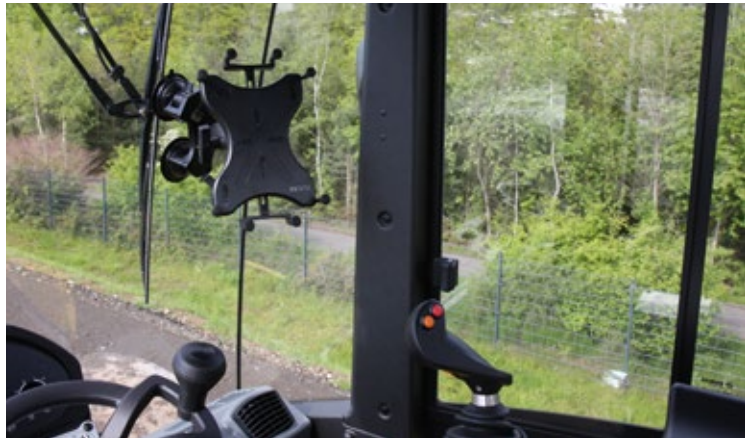
Quickly installed: The tablet holder can be conveniently placed anywhere in the cab using the quick-release fastener.
